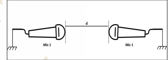
The two microphones are placed at a  $\overline{d=1m}$ . The two microphones are connected to the input channels of an oscilloscope.
